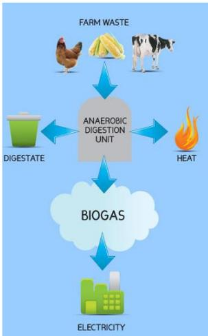
Anaerobic Digestion is a four part process converting organic waste to methane and digestate. During **Hydrolysis**, the organic waste is broken down into simple soluble organic compounds by enzymes similar to those found in the mouth. Through **Acidogenesis** these are fermented into intermediate products such as acetic acid.
